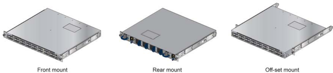
Figure 3-6: Improper Bracket Mount Example for Four-Post Rack Mount
